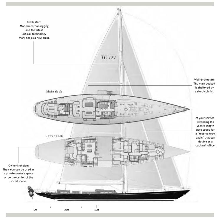
LOA: 127' 4" (38.8m) LWL: 91' 8" (27.95m) Beam: 25' 3" (7.7m) Draft: 14' 9" (4.5m) Displacement: 140 to
